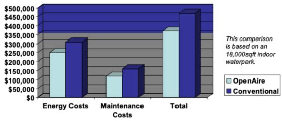
Based on analysis by JLC Hospitality and Andelman & Lelek Engineering an OpenAire structure can save over \$58,000 in Energy costs annually. Assuming that 25% of maintenance cost is devoted to maintaining the waterpark building, OpenAire's maintenance free structure offers a savings of \$40,000 annually.
